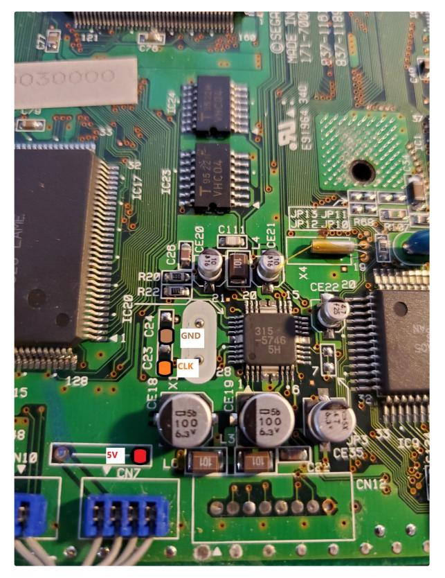
4. With the DFO now connected to the points previously used for the Crystal. You will have the S0 pad unconnected on the DFO board. Currently your console is either NTSC or PAL. However with the DFO you have the option to change that and also make it switchable. To do this locate the JP1 and JP2 jumpers on your console. They may be on the underside of the board.
