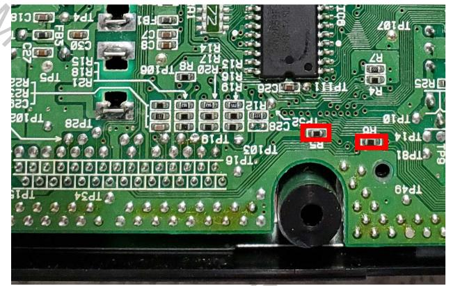
Optional 6. If you intend on enabling the Video Bypass, remove all components in red below.
