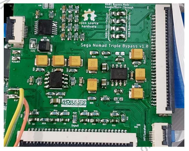
14. Now plug in all of the FFC cables to the QSBs, Main board, and Sub board. Blue plastic is always facing up for each connection.
