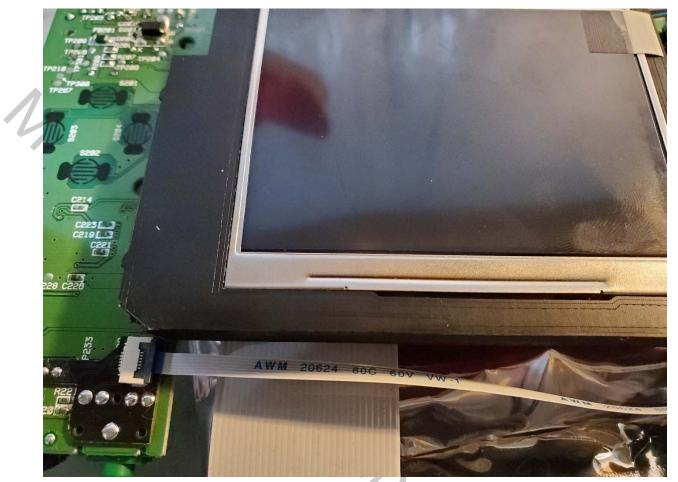
Optional 10. If you have chosen to perform the Video Bypass, install the AV-Out Board to the miniDIN as shown. The board should be as flat as possible. You may need to trim the ground pins on the MiniDIN. If you are going to be installing an aftermarket LCD screen, the pins have been labeled for your convenience.
