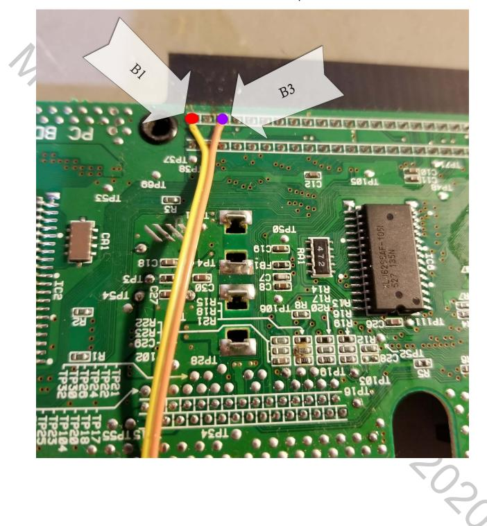
8. Connect the B1 and B3 audio lines to these solder points for the cart slot.
