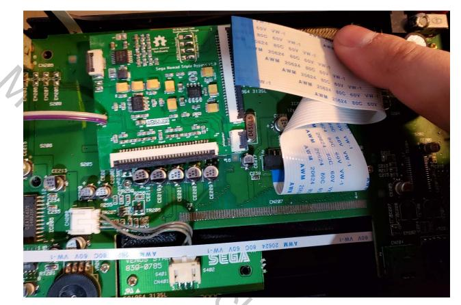
21. The Input 30pin FFC has no special requirements for installation. Just be certain that you did not cover any screw holes or pinch points on reassembly.
