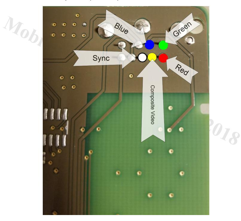
15. With all of the output connections made, you are done soldering. Clean up any flux or residue and double-check your solder joints. The last part is to reassemble the SSDS3. No special steps are taken here.
