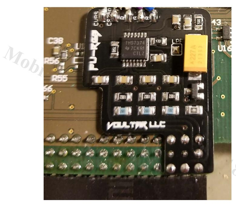
9. If you wish to set the Low Pass Filter to off, now is a good time to do so. Just remove the bridged solder points from the jumper labeled LPF. (It's recommended you leave this bridged for best results.)
