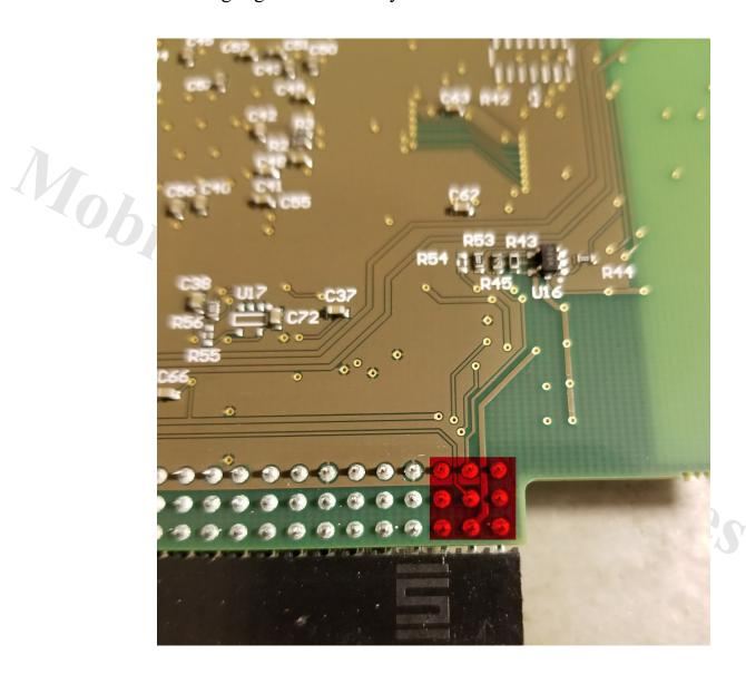
8. Solder the FU-RGB board in place. This should be very quick. Ensure that you are making a good connection with the pins.
